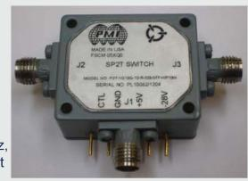
switching speeds of 40nsec, 25dB of isolation and 3.0dB of insertion loss typically. The DC current consumption is around 2.5mA at +5VDC and 2.5mA at -28VDC. The unit is offered in our compact housing that measures only 1.2"  $\times$  1.0"  $\times$  0.5".
